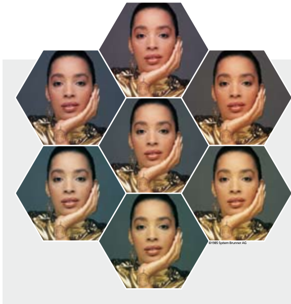
Dramatic colour fluctuations like those around the original (centre image) typically occur in 4c print production, even if solids are consistently uniform Photo: System Brunner
